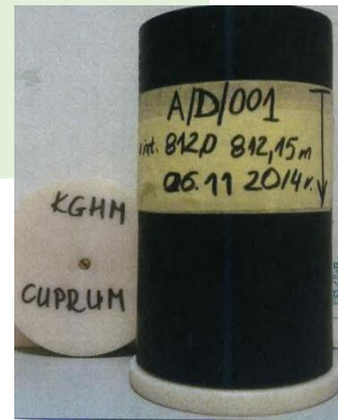
Container for the core sample for degassing
